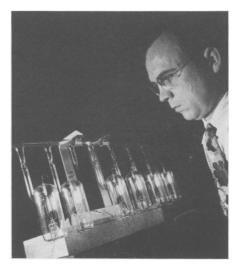
PLENTY OF NOTHING—The electronic gauges which are adept at measuring almost nothing, developed by Robert T. Bayard, can detect air in a vacuum where only one air molecule remains out of every 10,000 billion originally present. This device will aid in exploring regions of ultra-
