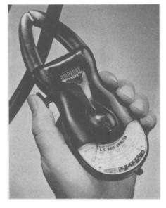
this 12-ounce pocket instrument, in a plastic case, features two insulated split-core transformer probes which are opened by a plastic trigger to close around conductors. Science News Letter, July 8, 1950
