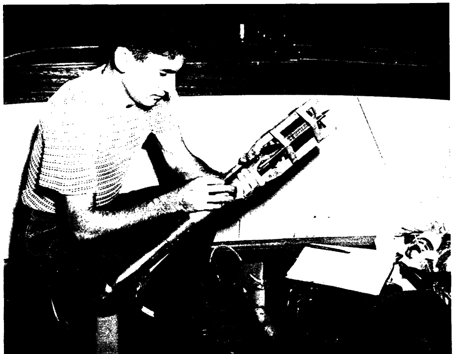
IT'S A BATHYTHERMOGRAPH! —This mechanism will help to disclose some of the secrets of the ocean's drifting "meadows," populated by minute marine creatures known as plankton. Everett C. Jones, one of the research team, is shown adjusting the educated gadget, which measures ocean depth and temperature.
