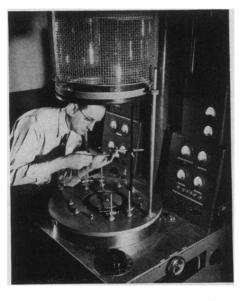
ONE AT A TIME—This clear glass sheet will soon become a mirror that "sees" and reflects only one color at a time—either red, green or blue. Demonstrated by Kenneth L. Fromm, the mirrors will be used at both the transmitting and receiving end of experimental color television apparatus.
