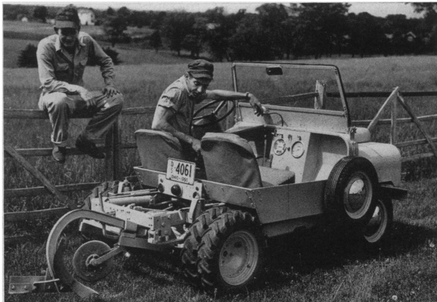
DOUBLE DUTY —This versatile vehicle is an answer to the farmer's need for a machine that will do a light tractor's work and provide transportation too. This photo shows a 10-inch plow mounted on a hydraulic lift. Harrow, cultivator and other implements are also available.
