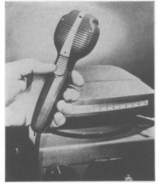
shown under the thumb in the picture, is pushed up the machine records. For playback the switch is pushed down.
