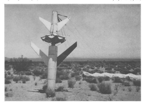
RECOVERY ASSURED—A free-falling body, after a drop of nearly seven miles, hits the earth. Its descent first checked by automatic dive brakes, shown open, and then by the parachute which is shown at the right, the body is buried nose first in the sandy soil of the California desert. The model wings are undamaged and the instruments and the records made during the fall are safe.
