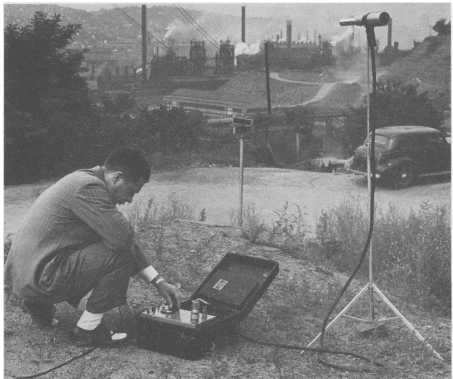
SMOG SAMPLER —The improved electrostatic sampler is used to trap all types of dusts, fumes and smoke in atmosphere. The instrument will be an important tool for investigation of air pollution causes by health officials and industrial hygienists. (See Next Page.)
