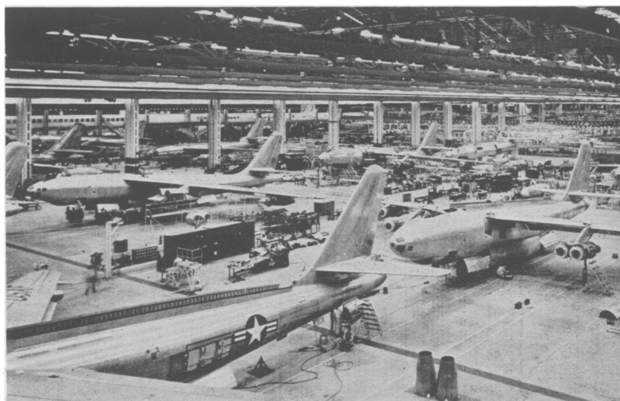
STEPPED UP PRODUCTION —Expanding activities in airplane plants, due to the world's unsettled conditions, are reflected in this Boeing plant at Wichita, Kans., where giant jet-propelled bombers for the Air Force are being made. Picture shows the B-47, 185,000-pound plane in the 600-miles-per-hour class. It is the Stratojet, an improved version of the plane that crossed the continent from Seattle to Washington, D. C., in three hours and 46 minutes.
