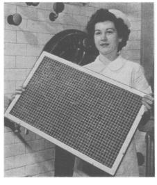
AIR FILTER for use in hot-air-heating and air-conditioning systems, shown in the picture, is made of plastics that become charged with static electricity when exposed in a current of air. This electric charge attracts even the finest particles of foreign matter in the air.
