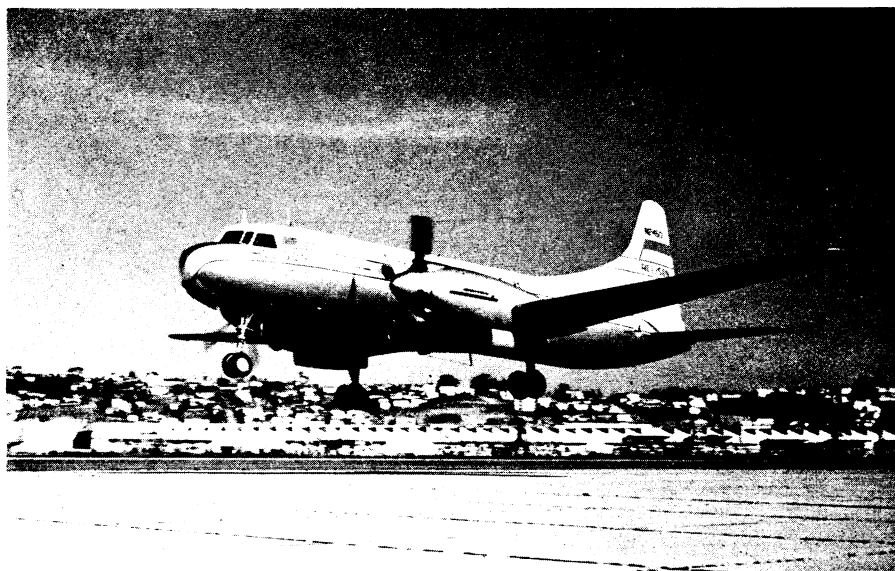
TURBOLINER —This is the first air liner to be equipped with Allison turbo-prop engines. The turboprop is similar to the turbojet, but instead of using the gases of a gas turbine directly for propulsion, they are used to turn a shaft and propeller.
