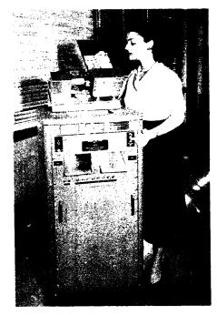
COUNTS MONEY—Worn-out paper money is put through this machine where an electric eye counts the bills. It can handle 30,000 bills per hour and rejects packages containing more or less than the correct number, 100.
