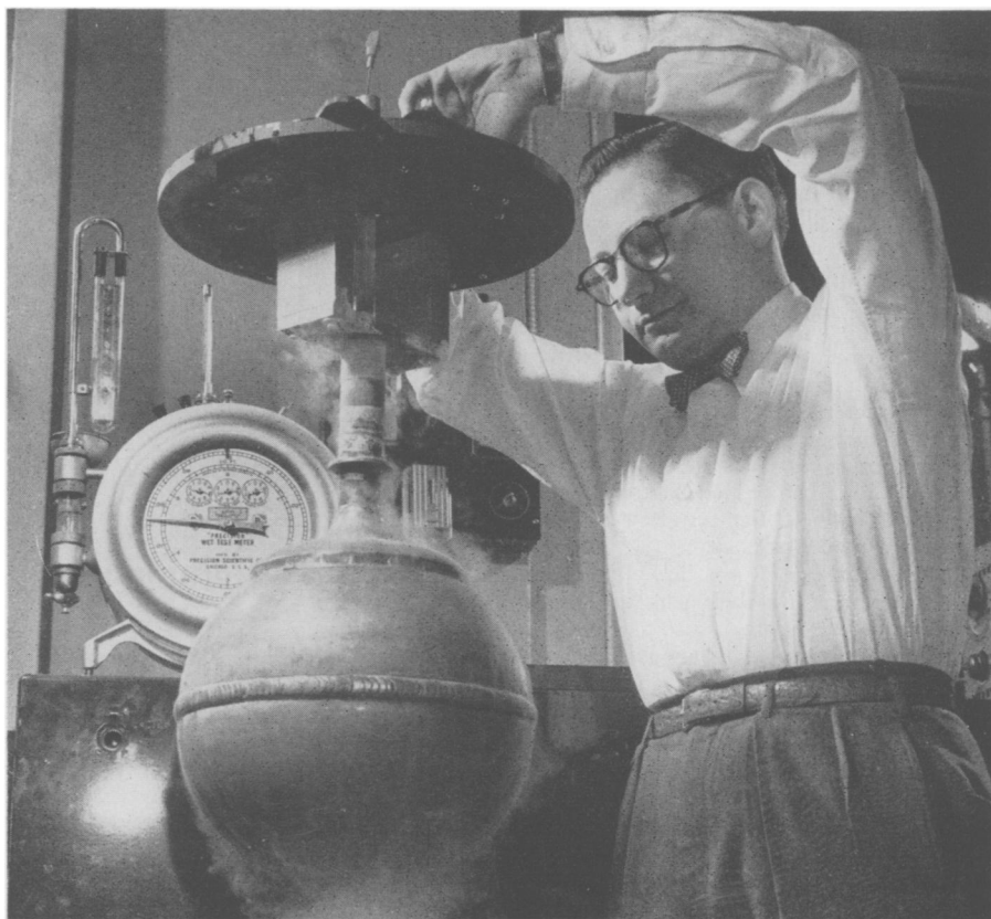
SUPER VACUUM BOTTLE —Keeping the world's coldest liquid is the job of this new vacuum bottle designed by Dr. Aaron Wexler of Westinghouse Research Laboratories. He is lifting the "bottle" from a bath of liquid nitrogen.
