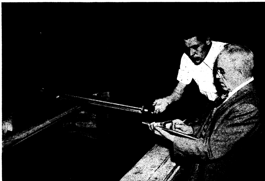
PROSPECTING TOOL —Dr. Louis B. Slichter, right, of the University of California's Institute of Geophysics and Fred R. Tesche use the "earth model" to record electrical "ripples" sent up by aluminum test sheet. Mr. Tesche helped design the equipment.
