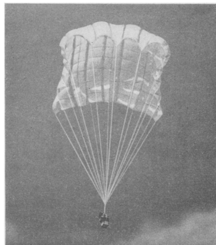
COTTON PARACHUTE —Square cargo chute made from strips of cotton muslin will replace the old rayon cargo chute. The unique strip design gives added strength to the new type chute.
