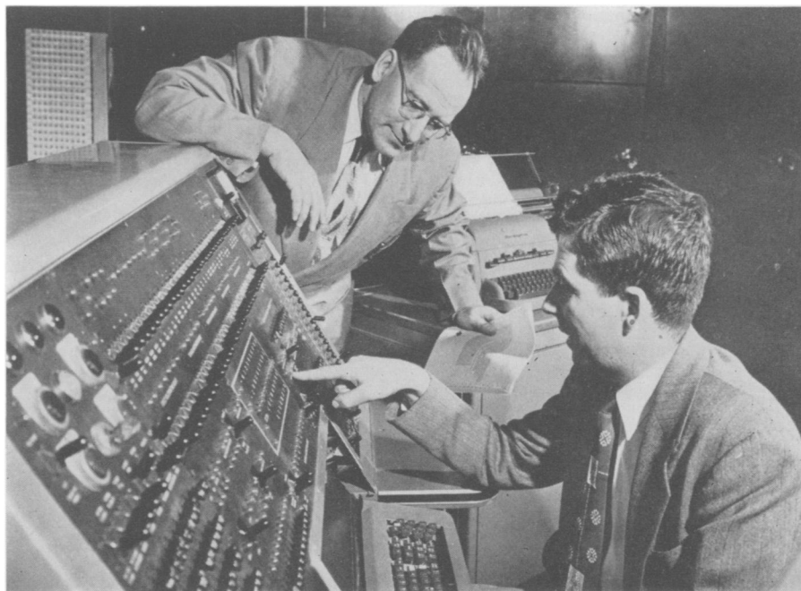
CONTROL BOARD —Closeup of the master control board of the UNIVAC. Dr. John W. Mauchly, one of the inventors, is leaning over the panel.
