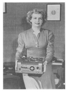
DICTATION MACHINE, shown in the photograph, is a portable wire-recording type which can be used also for transcriptions. It is a light compact unit that provides a clarity of voice reproduction. No erasing is necessary and the wire is used thousands of times without loss of fidelity.
