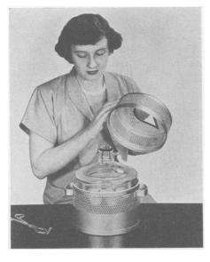
plosive action, is shown in the photograph. It is designed particularly for use with small vacuum desiccators in which drying is aided by vacuum. The upper part of the aluminum holder is perforated to relieve pressure; the lower part has a solid surface to catch spilled chemicals.
