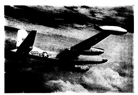
JET-PROPELLED LABORATORY—The nation's first jet-propelled "laboratory," now placed in operation for the high-speed flight testing of turbo-jet engines, is shown here in flight. The test engine is housed in the nacelle under the bomb bay. The plane is equipped with hundreds of special instruments which will record every phase of the test engine's performance in flight.
