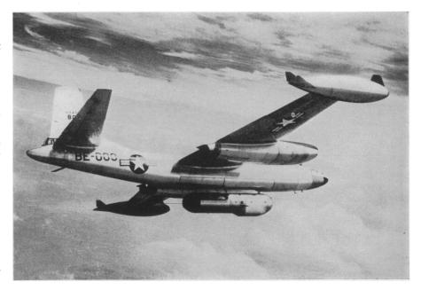
JET-PROPELLED LABORATORY—The nation's first jet-propelled "laboratory," now placed in operation for the high-speed flight testing of turbo-jet engines, is shown here in flight. The test engine is housed in the nacelle under the bomb bay. The plane is equipped with hundreds of special instruments which will record every phase of the test engine's performance in flight.
