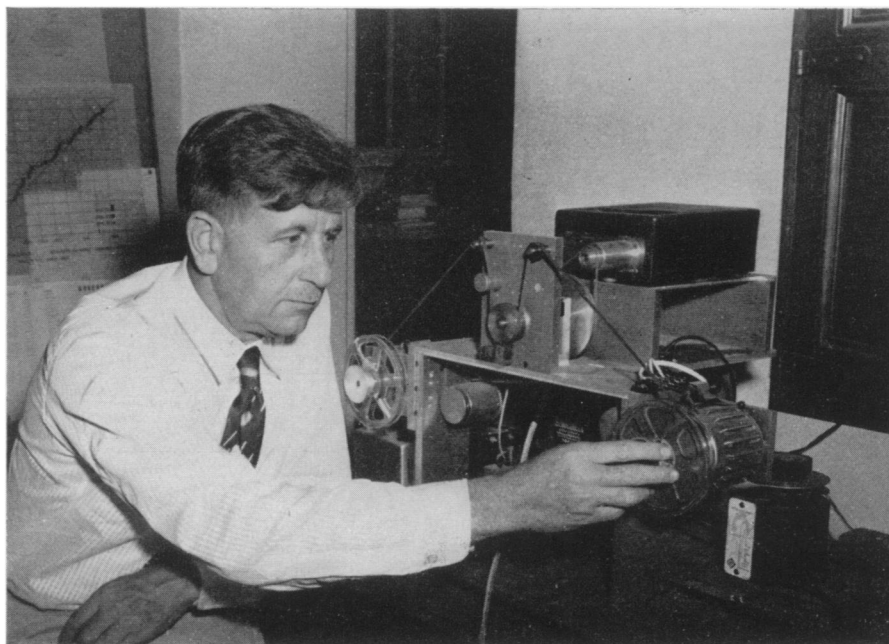
AUDIBLE EARTHQUAKES —Dr. Hugo Benioff is shown here with the seismic tape recorder he devised for continuously recording the different vibration frequencies of earth shocks.
