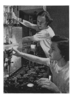
HYDROCARBON RESEARCH—By use of a platinum resistance thermometer and an extremely accurate resistance bridge, an accuracy within two one-thousandths of a degree Centigrade in freezing point comparisons of hydrocarbons is obtained at the American Petroleum Institute Laboratories in Pittsburgh.
