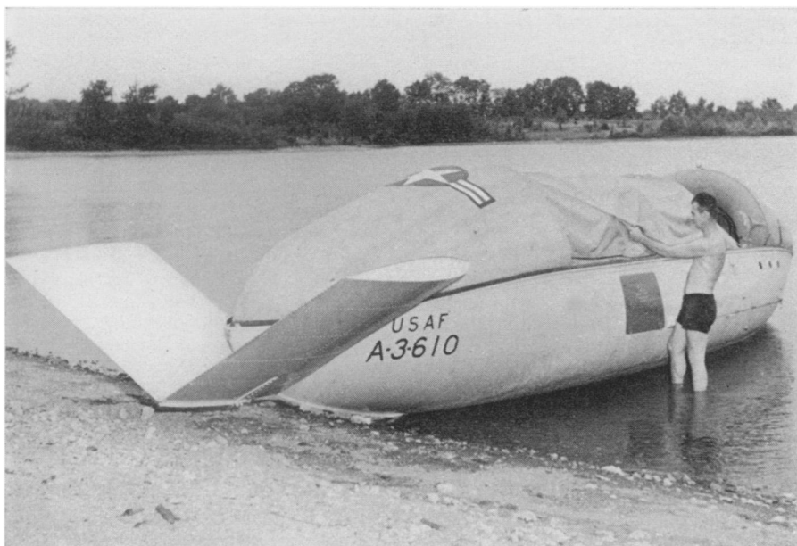
RADIO-CONTROLLED LIFEBOAT —The fin-like contraption on the stern of this radio-controlled lifeboat helps keep it upright when it is dropped by parachute. The fins are discarded by remote control after the boat lands in water and the craft is then steered to the side of stranded survivors.
