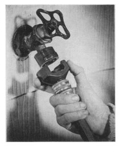
State GARDEN HOSE connector, for attaching the hose to a faucet, is made of cellulose acetate butyrate and is shown in the photograph. One part, with inside threads, screws directly on the faucet, and the other part, with outside threads, screws into the receiving end of the hose. A quick halfturn attaches the hose to the faucet and releases it.
