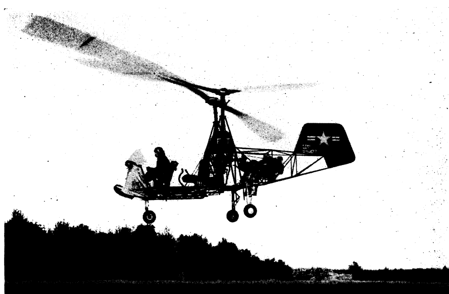
FIRST TURBINE HELICOPTER —The world's first turbo-rotor helicopter is shown on its initial flight. It is a Kaman Aircraft K-225 helicopter powered with a Boeing gas turbine. Marked increases in the plane's performance, because of weight savings, are predicted.
