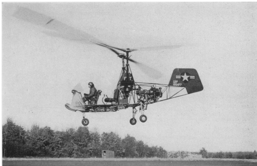
FIRST TURBINE HELICOPTER —The world's first turbo-rotor helicopter is shown on its initial flight. It is a Kaman Aircraft K-225 helicopter powered with a Boeing gas turbine. Marked increases in the plane's performance, because of weight savings, are predicted.
