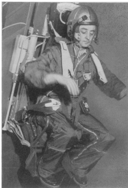
PILOT EJECTOR —The pilot's seat belt is automatically unfastened five seconds after he and the seat are ejected from a fast plane. Here the belt unfastener is demonstrated.
