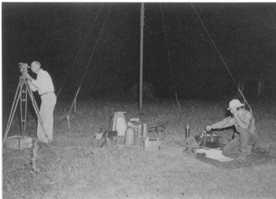
OPERATION FLARE —A rapid method for control surveys to supply basic data for mapping and field artillery fire control using airborne stations, equipped with signal lights and flares, has been worked out by the Engineer Research and Development Laboratories at Fort Belvoir, Va. Spotted at known and unknown points, simultaneous readings of the target's horizontal angle are taken with theodolites, equipped with recording cameras.
