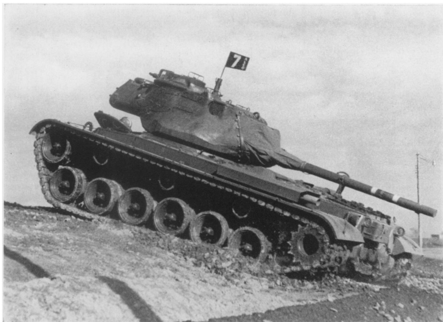
MANEUVERABLE TANK —The M-47 mounts an embankment showing its deadly 90mm, high-velocity gun which is operated by two separate electro-hydraulic fire control systems. "Many hundreds" of these new tanks are being readied for shipment to troops.
