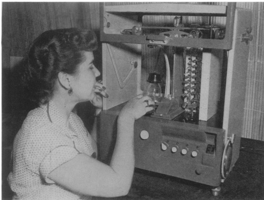
MORE SENSITIVE BALANCE —Miss Bunny Geisbert of the National Institutes of Health staff here shows how the newly developed balance, 10 times as sensitive as conventional projection balance, is operated.
