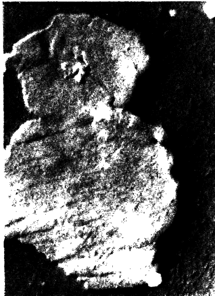
DIRECT POSITIVE IMAGE— A shadowed electron micrograph, printed directly on reversing photographic paper, shows the platelets of carbide, or cementite, that have been extracted from steel, magnified 40,000 times. The replica surface is the reverse of the steel surface, the depressions being actually projections on the original specimen.
