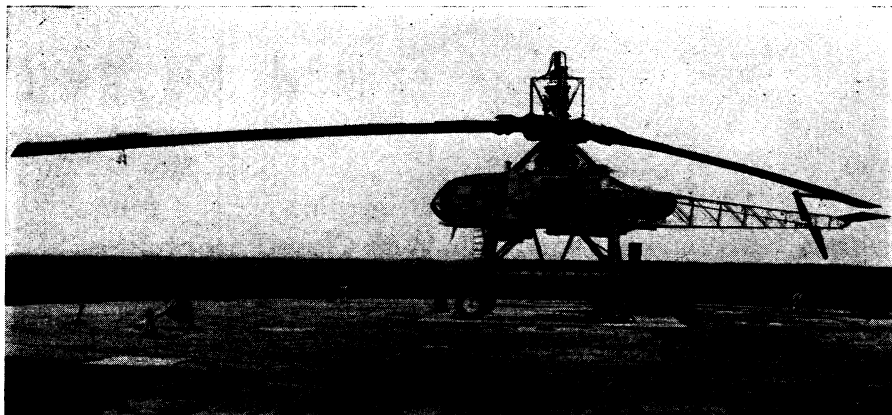
LARGEST HELICOPTER —The world's largest helicopter is now undergoing "tie-down" tests at Hughes Aircraft Company airport in Culver City, Calif. Known as the XH-17, it is powered by two turbojets and designed for short-range moving of heavy military equipment.
