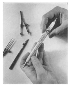
slide-rule scales are printed on the pencil barrel. Three sliding scales are printed on a transparent tube which slips over the barrel. The plastic pocket clip doubles as an indicator.
