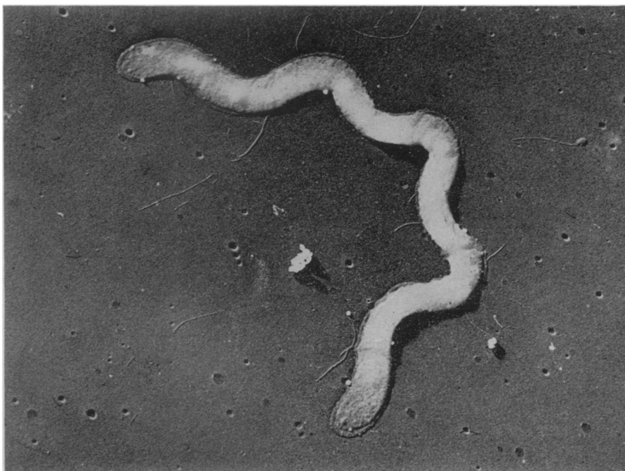
AIR-DRIED MICROORGANISM —Squashed into a two-dimensional sine wave, by ordinary air-dried preparation, the organism shown here is used as a test object in a new technique for electron microscopy.
