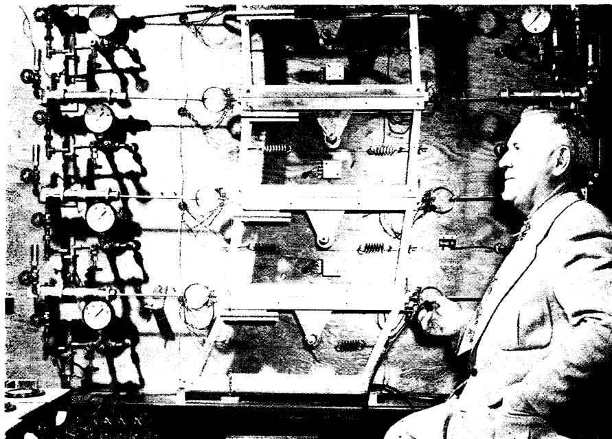
H-BOMB BLAST EFFECT —This model of a four-story building, represented by the four metal frames, is used at Stanford University to test the effects of bomb blasts on construction. The bent steel frames would, in reality, be twisted wreckage. Air-driven pistons can be adjusted by Prof. Lydik S. Jacobsen to represent the blast pressure of different bombs at varying distances from the building.
