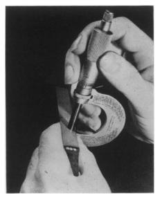
to .009 inch, as shown in the photograph. Especially useful in hard-to-reach places, the files can serve as go-or-no-go gauges during maintenance of delicate, high-speed machinery.
