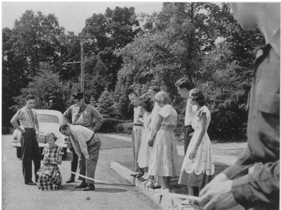
QUICK-STOPPING TEST —High school students, under the direction of Pennsylvania State College scientists, measure accurately the reaction time and the stopping distance of a test car through the use of a detonator device. A blank cartridge fires a chalk mark on the street at the start of the test and at the time the brakes are applied, making it possible to measure the danger zone in front of the car.
