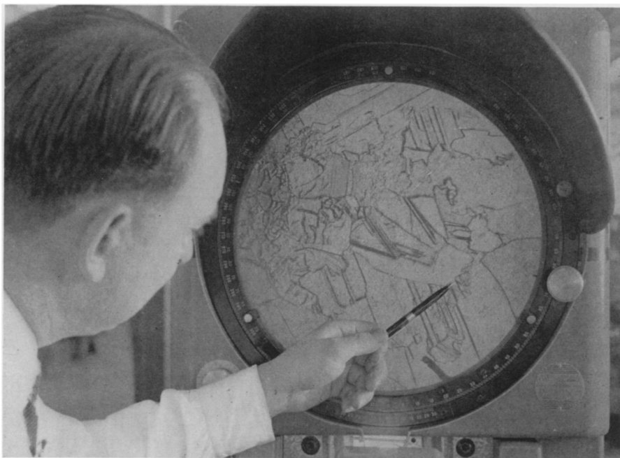
GERMANIUM WAFER—Magnified 20 times on a special contour projector, a germanium wafer looks like this. The black lines are the boundaries of single crystals of germanium.
