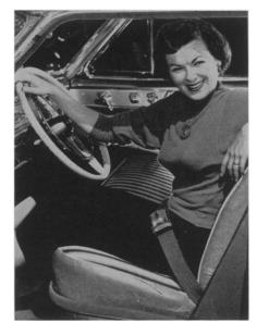
be fastened in about five seconds. Attached to the car chassis, the belt's webbing comes in various colors to blend with the car's color scheme.
