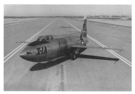
FOR 1,700 MILES PER HOUR—Scheduled to undergo flight tests at speeds over twice that of sound is this Bell X-1A. It is slightly larger than the X-1, the first United States supersonic airplane that crashed through the sonic barrier in October, 1947. It is rocket-powered with a liquid oxygen and a special alcohol-water mixture for fuel.
