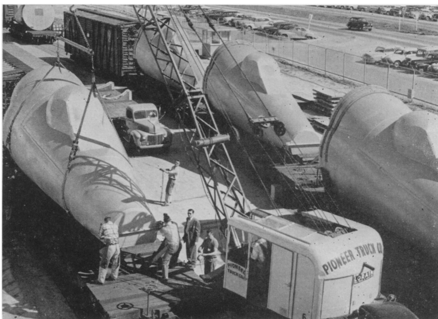
GIANT FUSELAGES —Shown being loaded for shipment from the Ryan Aeronautical Company yards at San Diego, Calif., these five giant aft fuselage sections are for the Boeing C-97 Stratocruiser, which can be used as a cargo carrier, a flying ambulance or an aerial tanker.
