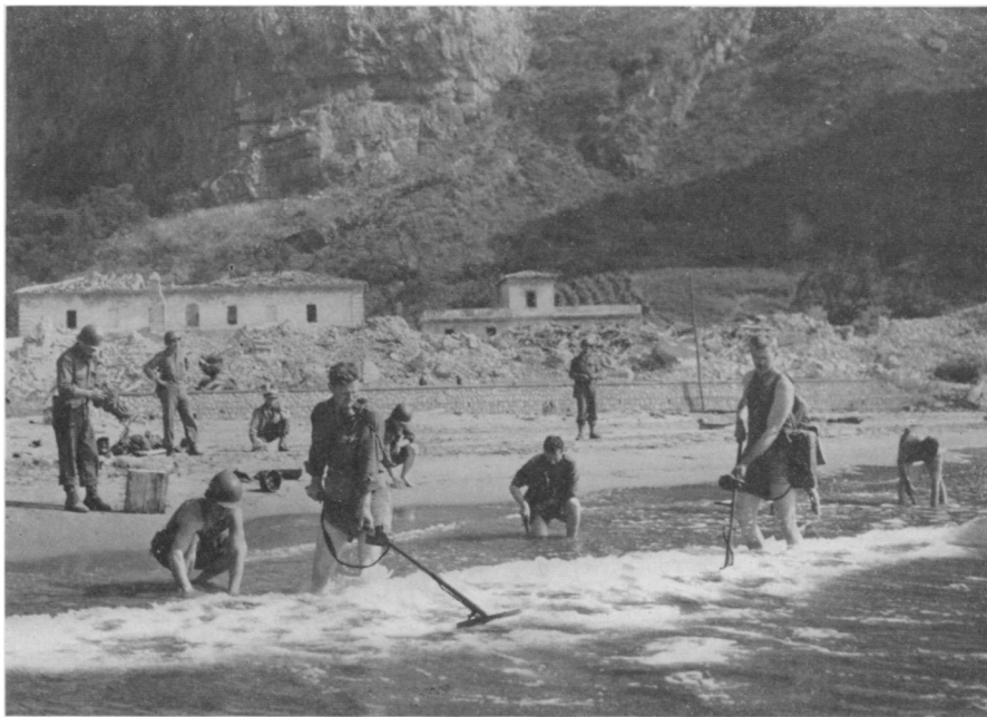
MINE DETECTOR —Discovered as a result of publication of the information by the National Inventors Council during World War II that a land mine detector was needed, the instrument had originally been developed for discovering buried treasure. This simple gadget, shown being used during the war, saved thousands of soldiers' lives and permitted rapid advances over mine fields.
