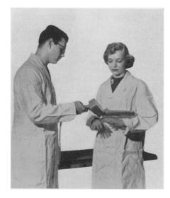
ALPHA COUNTER, shown in the photograph, checks large areas quickly for possible radioactive contamination. Operating on ordinary 115-volt, 60-cycle current, the device causes a loudspeaker to "pop" whenever an alpha particle is detected.
