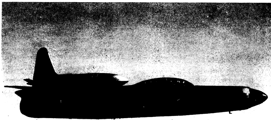
STARFIRE'S NEW LOOK —Plastic surgery has given a new shape to the nose of Lockheed's F-94C Starfire jet interceptor. The change-over increased air speed five miles an hour.
