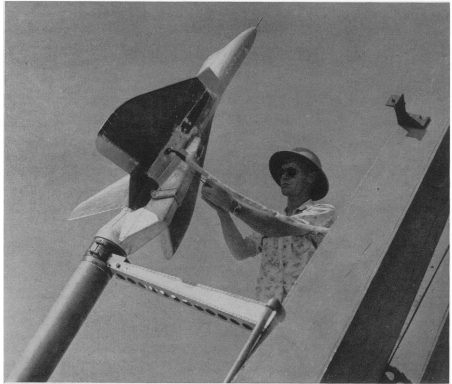
LAUNCHING MODEL —This dynamic scale model of a new jet fighter, the Navy's F4D Skyray, was fired into the sky for a supersonic test flight to investigate drag, stability and control.
