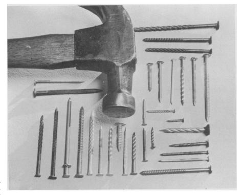
BETTER HOLDING NAILS—The right nail for the job is the goal of nail designers. Shape of head, shank, point, material and size all vary according to the nail's function. The threaded-shank nails shown in the photo hold harder the longer they stay in the wood.
