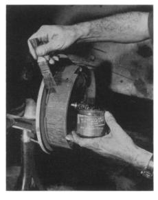
compound helps dissipate high heat created in the brakes during sudden stops. Truck, bus, taxi, and racing-car tests reveal the compound waterproofs linings, doubles brake life and eliminates frictional squeals. Science News Letter, July 4, 1953
