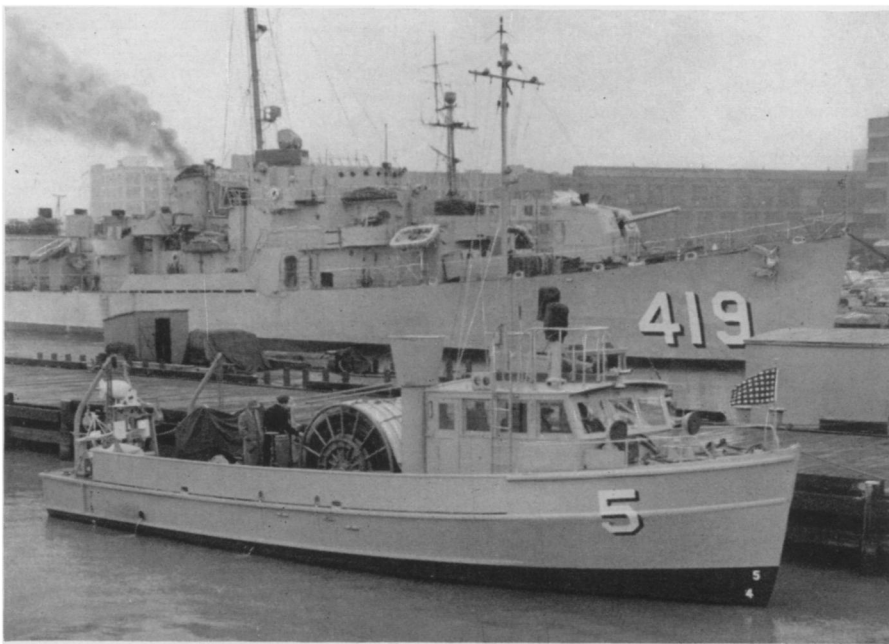
BABY WOODEN MINESWEEPER —The salty little craft shown in the foreground is the Navy's new 57-foot MSB 5. The large reel amidship carries heavy electric cable for magnetic minesweeping operations. The baby minesweeper can be manned by seven enlisted men who will spend most of their time aboard a larger ship still in design stages.
