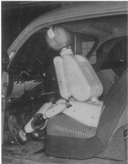
AUTO CRASH DUMMY — This artificial figure has been developed at Cornell Aeronautical Laboratory to simulate how human bodies react in automobile crashes.
