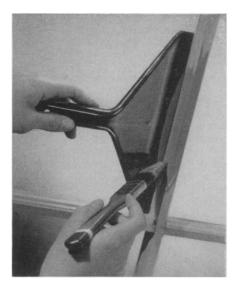
as shown in the photograph. Example: When the painter is coating walls, the handheld butyrate plastic device keeps paint off door jambs and baseboards. Small pads beneath it prevent streaking when the tool is moved to a new position.
